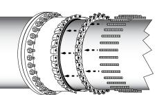
**Step 9** • Tighten nuts on all-thread-rod evenly, alternating to diametrically opposite position at approximately 20 ft-lbs increments to the recommended torque per AWWA C111 see table below. Two wrenches will be required. 9
