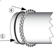
**Step 6** • Slide the FC400RG-PVC on to the pipe. Position the pipe and flanged coupling against the mating flange, inserting the flange gasket between the flange faces. Assemble the flange joint using flange bolts.
