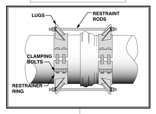
**Step 1** • Assemble the pipe joint or coupling per manufacturer's installation instructions.
